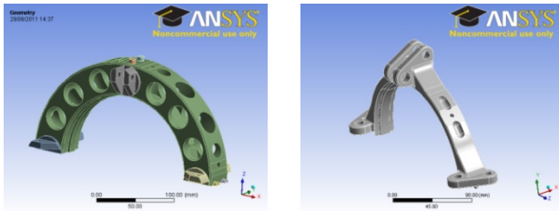
Figure 2: current collar design (left) and new collar design (right) for S3F fixed point.
